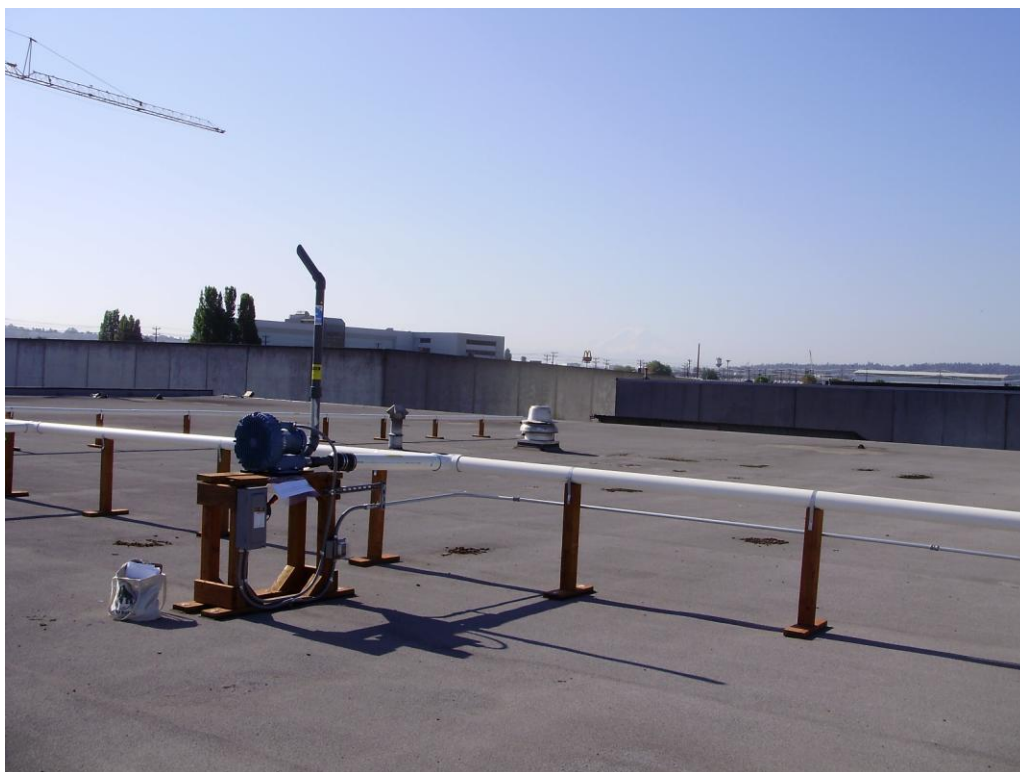
Photograph 12: Blower and stack looking south. Air intake is approximately 40 feet away.
